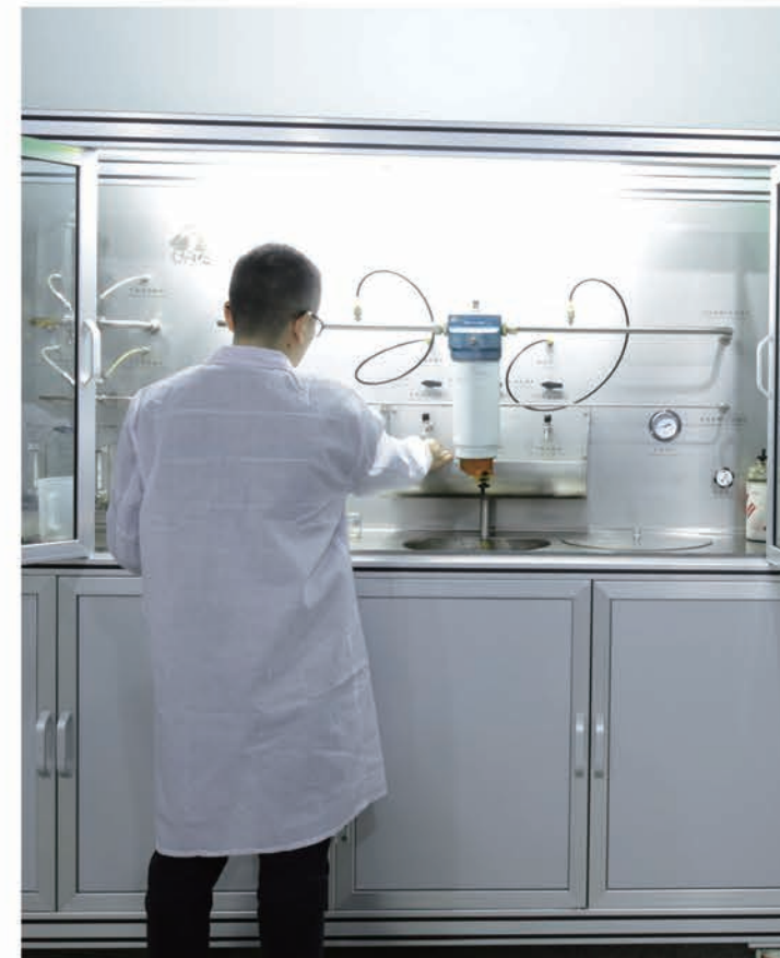
燃油滤清器油水分分离效率试验台 FUEL FILTER OIL-Water Separation Test Bench
